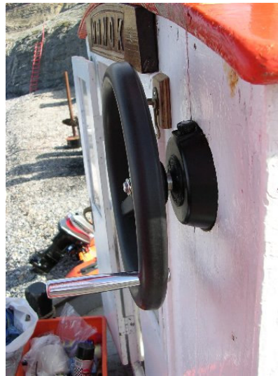
Outer steering wheel on the wheel house.
