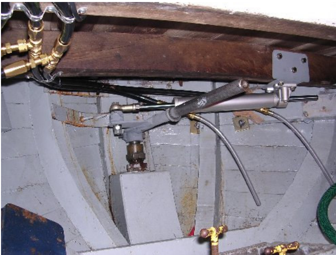
The hydraulic steering system is mounted.
