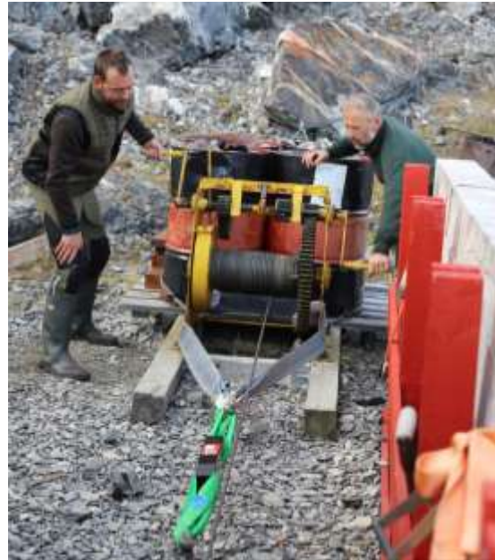
Left: Strindberg Land. Red mark: Nordfjordhuset. Blue mark: Location at Holmesø. Right: Measuring the necessary tractive force for heaving "Agsut" on shore.
