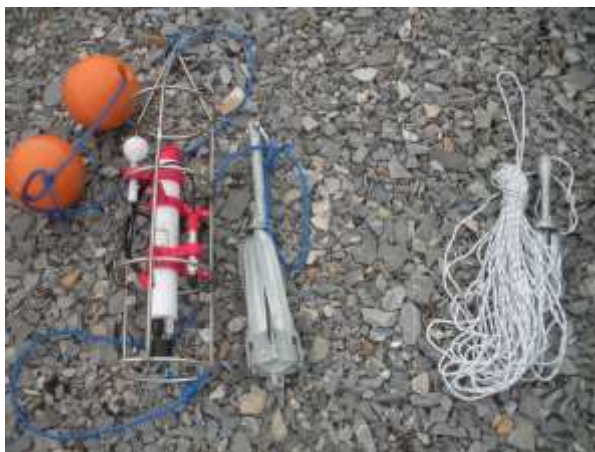
Left.: Example of underwater buoy measuring light, temperature, pressure, salinity and chlorophyll all year round on the three localities. Right: Søren prepares CTD for oceanographic testing along the sections throughout the fjord.
