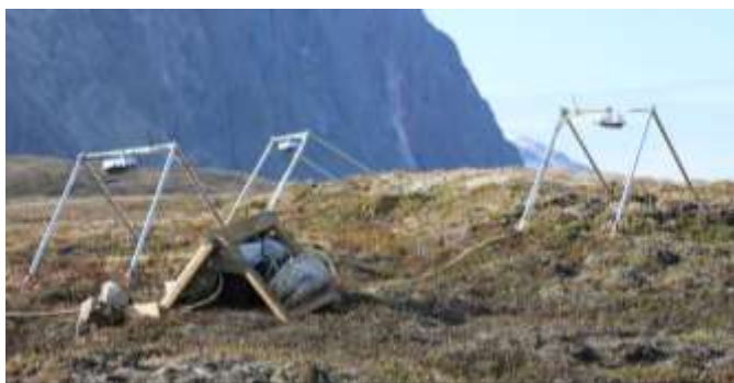
Toke's automatic cameras for monitoring of plants and insects on land.
