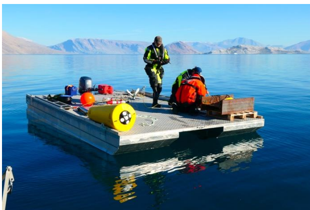
GIOS underwater instruments are acoustically triggered and come to the sea surface after measuring for a year. New instruments for the next season are deployed. Photo Søren
