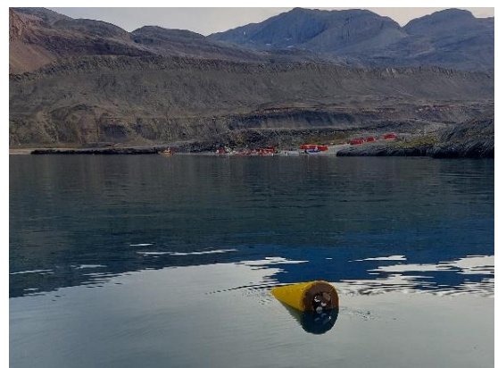
GIOS underwater instruments are acoustically triggered and come to the sea surface after measuring for a year. New instruments for the next season are deployed. Photo Søren
