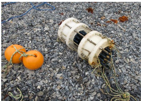
The water sampler worked perfectly. Water isotopes are now collected in the fjord all year round. Photo Søren
