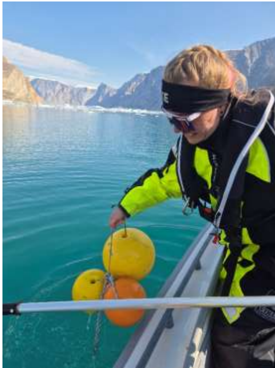
Nanna deploys incubation bottles to measure primary production in the fjord. The bottles are attached to a line with floats so that they remain suspended in the water column under in situ conditions and can be used to determine phytoplankton primary production.
