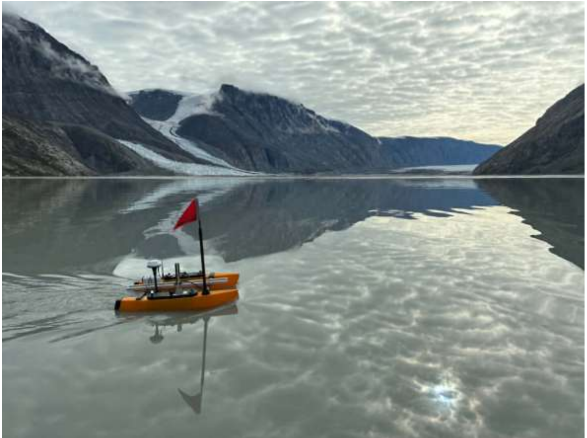
Measuring discharge from Rhedin Fjord using an unmanned surface vessel equipped with an ADCP.
